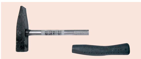
Figure 15: RAPEX notification no. 0125/06 deals with a hammer where the handle breaks.
